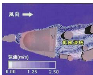
Results of analysis of wind conditions due to prevailing winter winds (plan)
